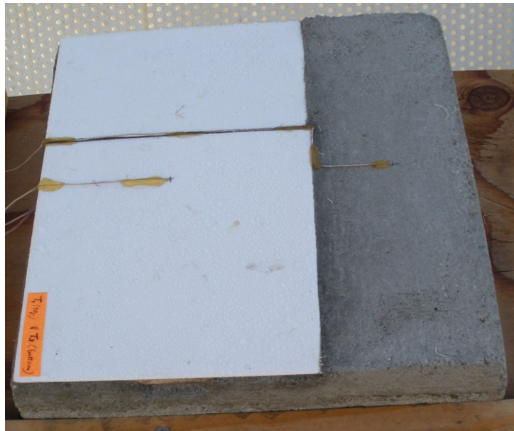
Figure 3: test plate for thermal test
