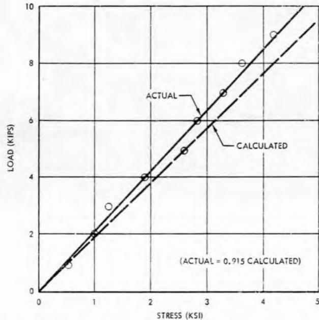
Fig. 12—Tower-leg stress graph, south (tension) leg
