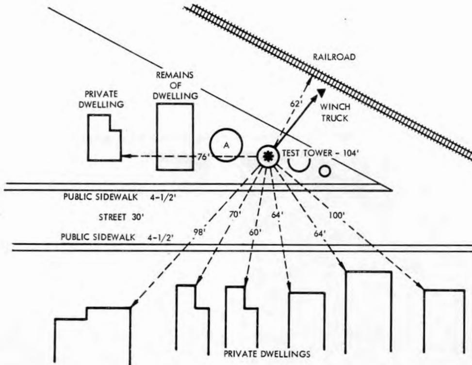
Fig. 5—Plot plan of test-tower site
