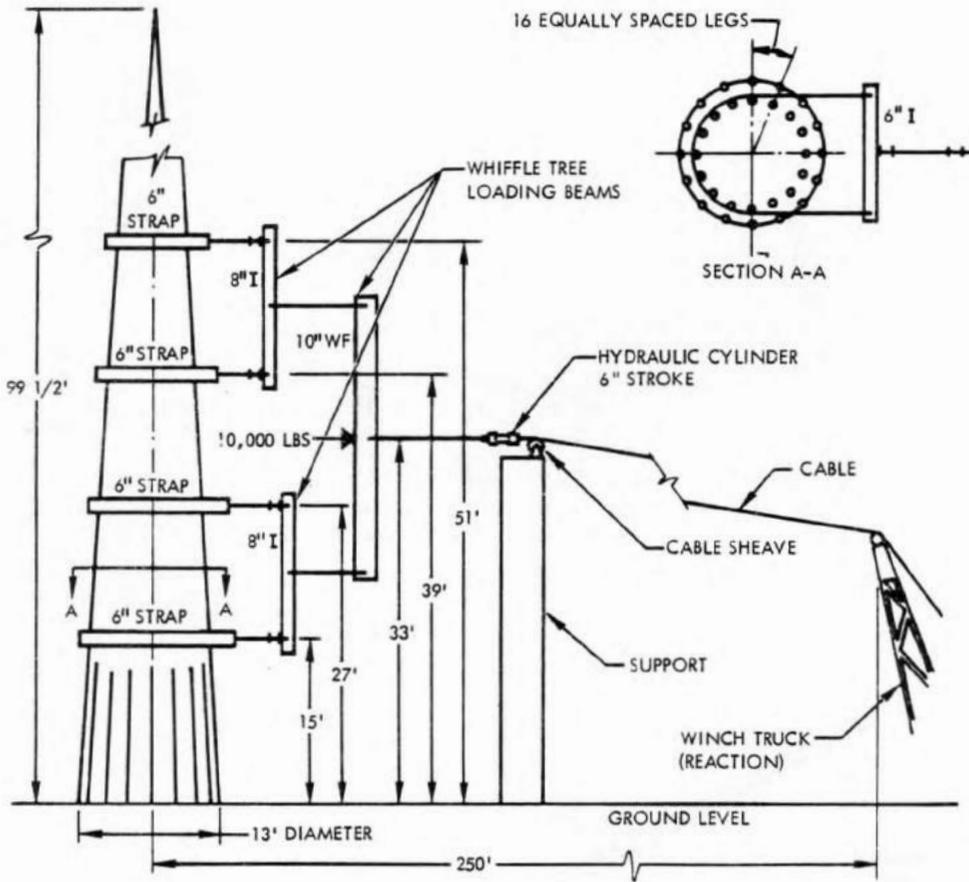
Fig. 6—Schematic of test setup
