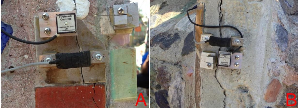
Figure 2.3: (A) North and (B) south side crack displacement sensors
